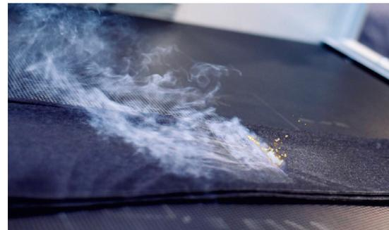
Laser finishing process being performed on jeans.
