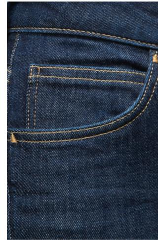
Examples of the use of bar tacks and embroidery techniques to replace the use of metal rivets.
