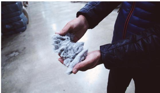
Jeans have been collected and are being shredded and turned into post-consumer recycled fibres.
