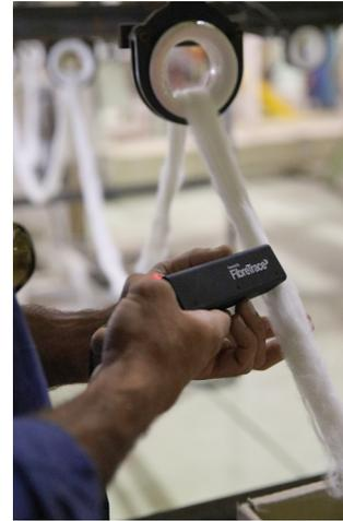
Cotton fibres being scanned using FibreTrace® technology.
